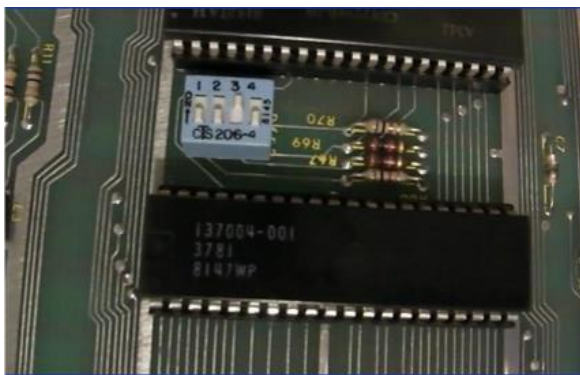
Figure 2 - Dip switch configuration for Tempest
